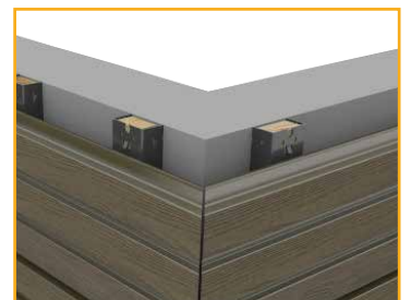
Mitre cut external corners. Allow for expansion gaps.
